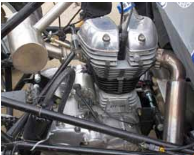
The India Enfield EFI500 air cooled single cylinder engine.
