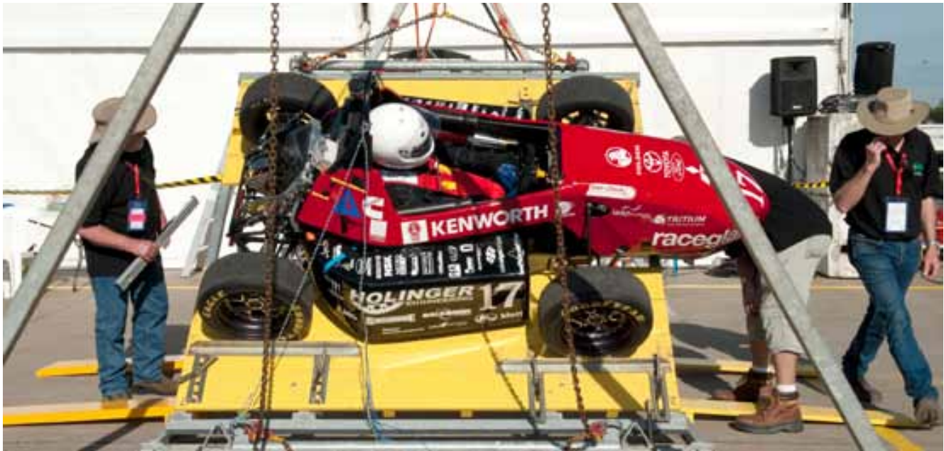
Swinburne's electric car passed the tilt test - one of the rigorous safety checks conducted before vehicles are allowed in the dynamic events.
