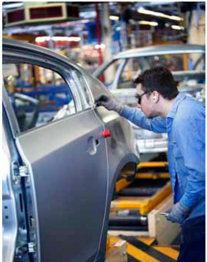
Doors on the Cruze incorporate triple-layered sealing to reduce noise, vibration and airflow through the door and into the passenger compartment.
