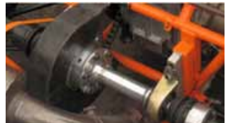
The straightforward spool drive system fitted to the University of Newcastle car.
