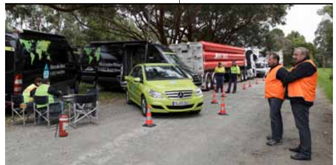
An interesting aspect of the Mercedes Benz F-CELL World Drive project was the logistics involved in delivering the Hydrogen fuel to the teams. The Linde Group (BOC in Australia) provided global support with mobile tankers.
